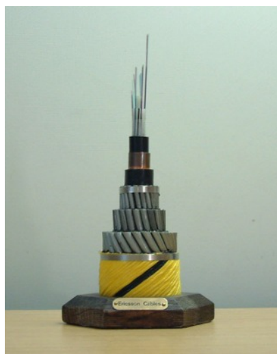
Section of a submarine cable,
